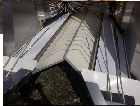
Soft-Catch Material (elastomeric polymer)
